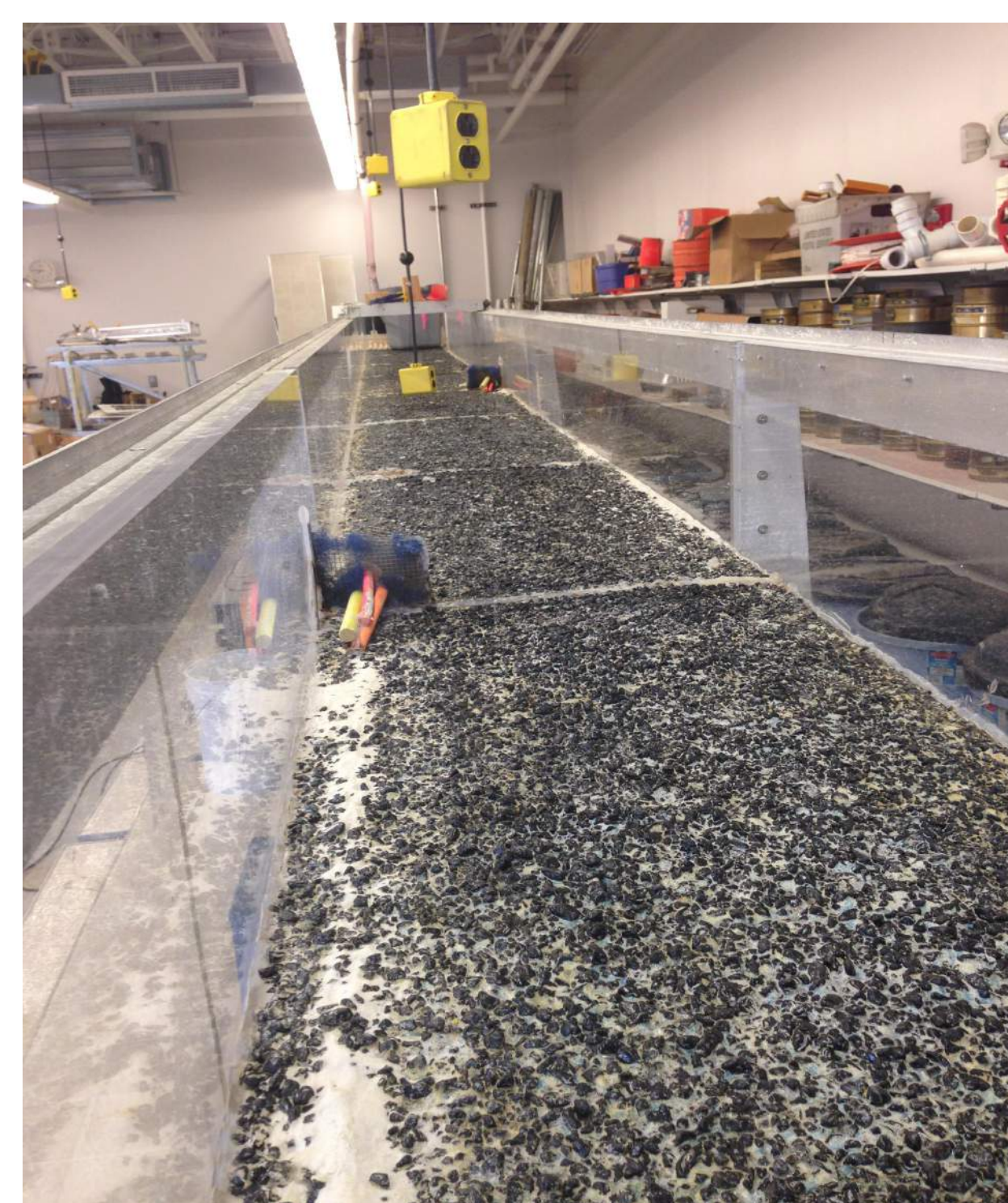
15 by .6 meter flume. Flow direction is towards camera
