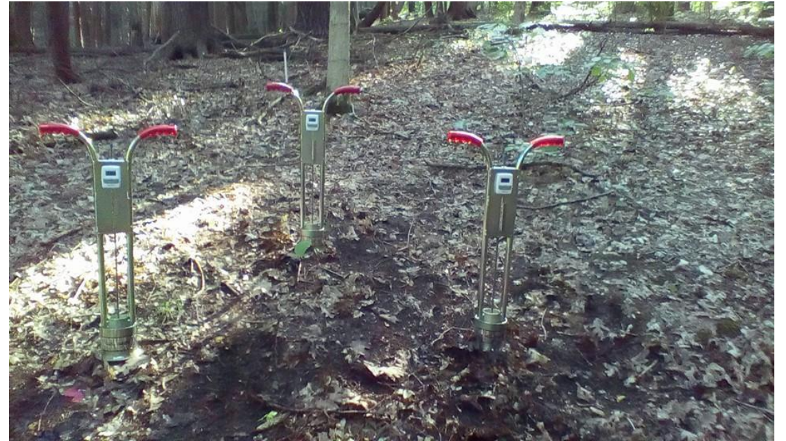
Infiltrometer set up with three replications in a 1 m triangle.
