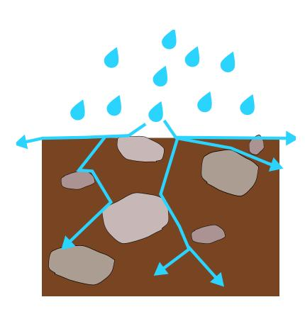
Plot showing differences in runoff rate due to both slope material and gradient (above). For soil-mantled sites, runoff volume increases with slope gradient, while boulders do not yield runoff even on high slopes. (Left) Schematic diagrams showing observed flow paths for both surface cover endmembers.
