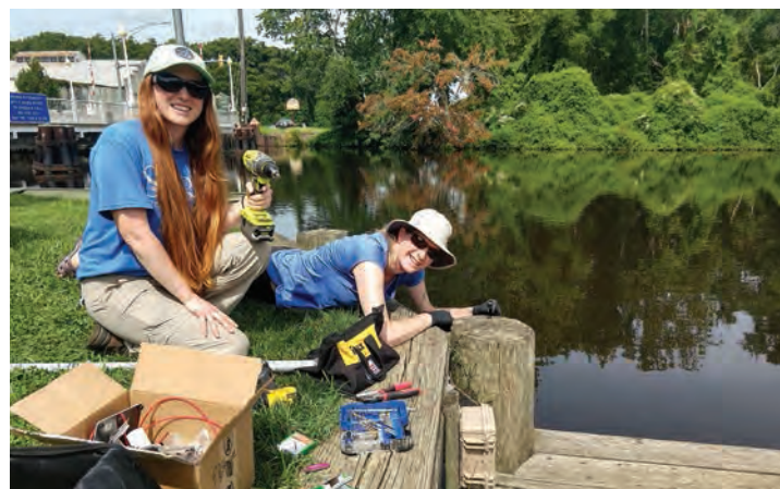
Rachel Johnson and Shannon Hicks install an EnviroDIY™ Monitoring Station in the Pocomoke River in Maryland to track sediment pollution.
