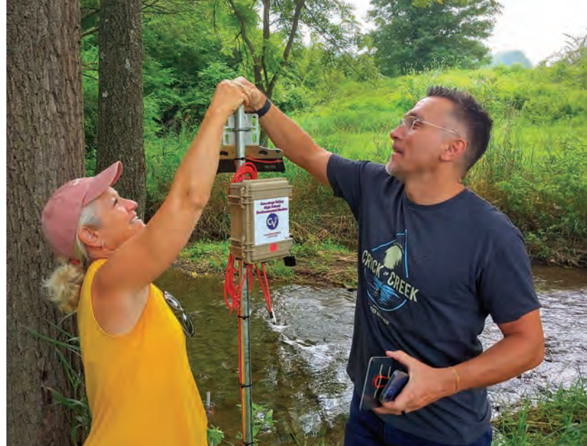
Kerri Snavelly and Jim Hovan, Conestoga Valley High School science teachers, install an EnviroDIY™ Monitoring Station on Stauffer Run at the Lancaster County Country Club.
