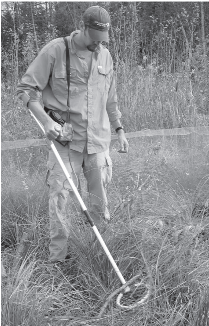
FIG. 1. Using a PIT-pack to search for PIT-tagged, recently metamorphosed Rana pipiens in a terrestrial enclosure in a three-year old clearcut in Maine, USA. We held the transceiver in a shoulder bag, and constructed the antenna using a modified forearm crutch for ergonomics. We varied the angle of the antenna to increase the detection probability as we searched for concealed frogs, and an audible beep from the transceiver alerted us to detection of a tag. Photograph by Valerie Moreau.
