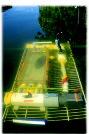
An underwater chamber for measuring the impact of a paper plant's discharge on the oxygen supply of the Flint River.
